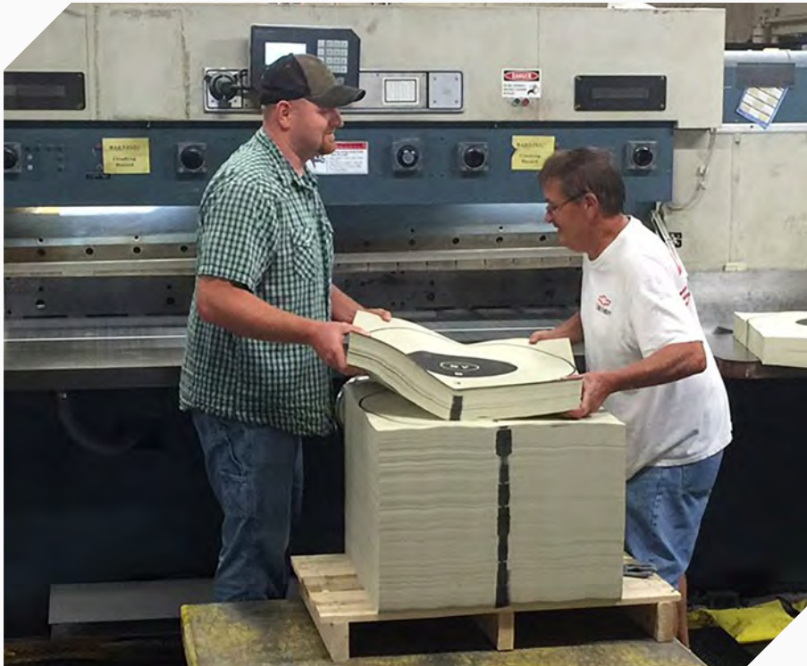
Document Services employees cutting out targets with the large paper cutter at Rock Island Arsenal.
