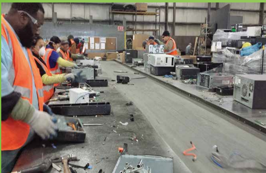
The Regency Technologies "triage line", in Twinsburg, OH, where material is initially taken apart and segregated.
