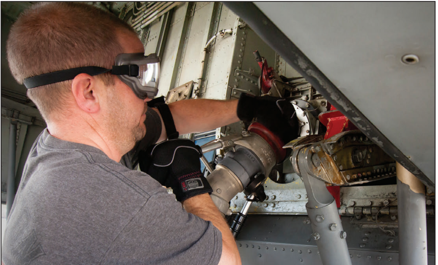
Tech. Sgt. Thomas Conroy, 459th Aircraft Maintenance Squadron crew chief, attaches a fuel line to a KC-135R Stratotanker prior to refueling on the Joint Base Andrews, Maryland, flight line July 20. The KC-135 is an aerial refueling aircraft capable of holding up to 200,000 pounds of fuel. U.S. Air Force photo by Tech. Sgt. Kat Justen
