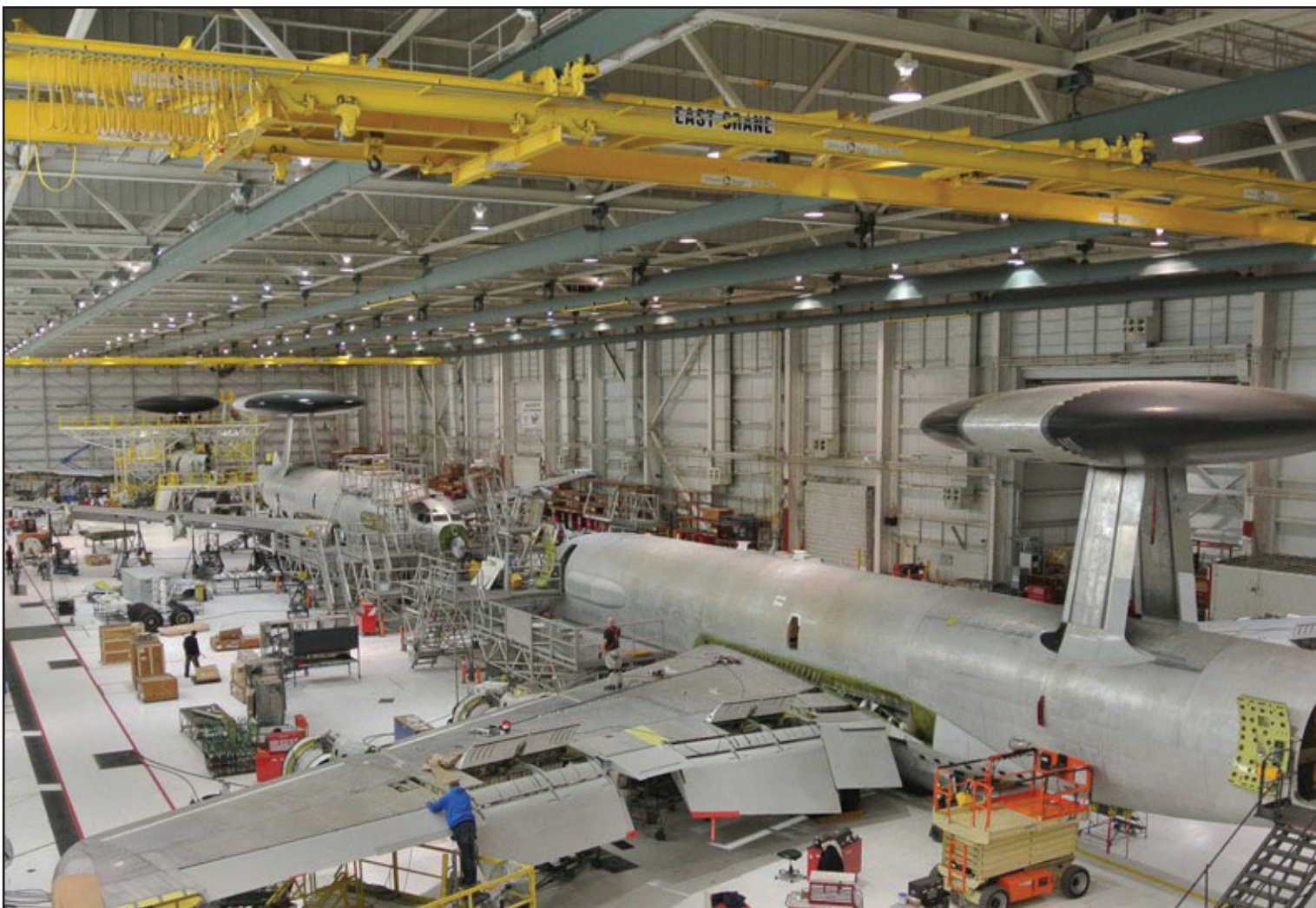
Workers at Tinker Air Force Base, Oklahoma, install critical 40/45 upgrades to E-3 AWACS aircraft during programmed depot maintenance at the Oklahoma City Air Logistics Complex. Defense Logistics Agency Energy recently awarded an energy savings performance contract to implement energy conservation measures at the OC-ALC. U.S. Air Force photo
