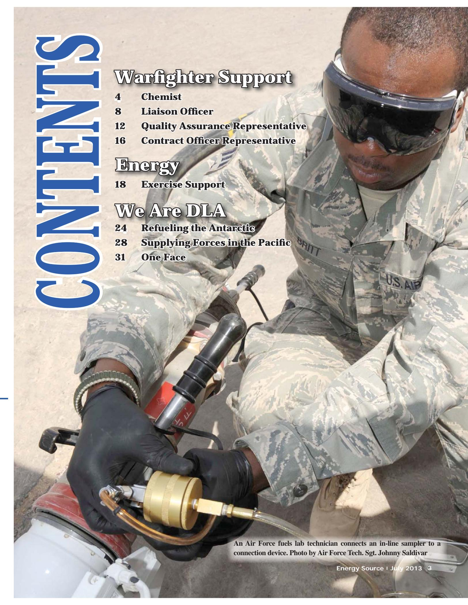
An Air Force fuels lab technician connects an in-line sampler to a connection device. Photo by Air Force Tech. Sgt. Johnny Saldivar
