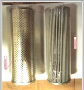
The government ordered the filter on the right, but Kustom delivered the unauthorized substitute filter on the left which is clearly dissimilar to the required item. (Courtesy photo)
