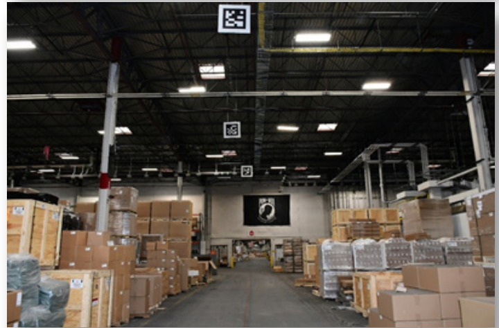
Quick response codes, suspended from the ceiling at DLA Distribution Susquehanna, Pennsylvania's Eastern Distribution Center, provide fiducial targets for the Automated Guided Vehicle from a pre-programmed route that directs the AGV from receiving to storage, out loading and then back.
