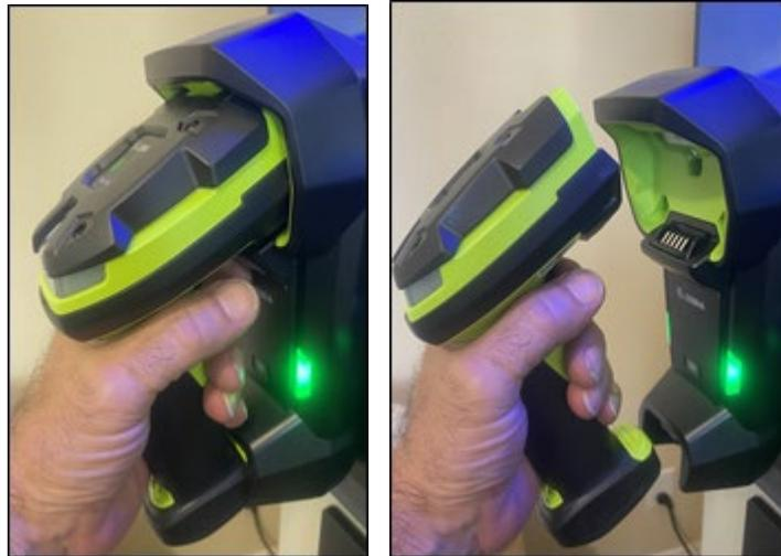
*Figure 3-15 – Grasp scanner firmly then pull from cradle*
