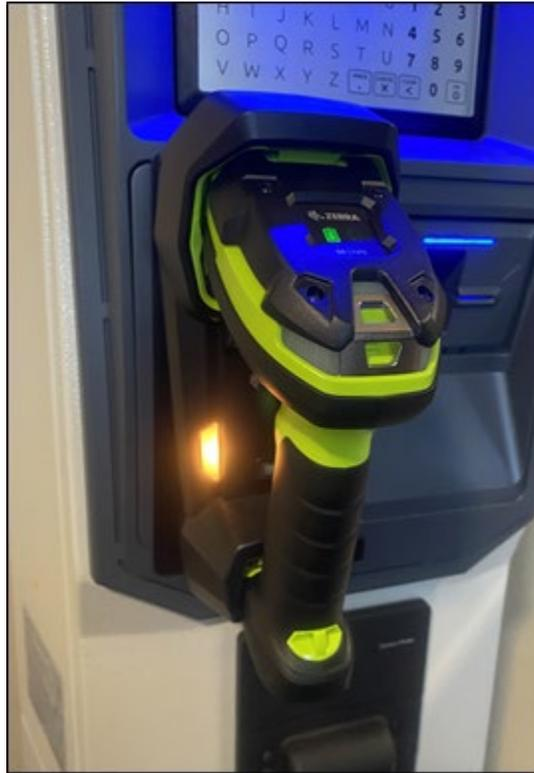
*Figure 3-14 – External Scanner mounted on Fixed Device*
