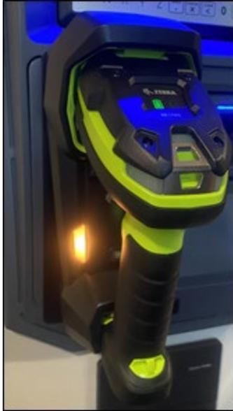
*Figure 3-17 – Replace scanner in cradle (will glow yellow as it charges the scanner)*
