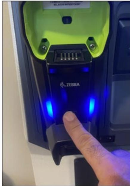
*Figure 3-22 – To page the scanner, press the Page button on the cradle*
