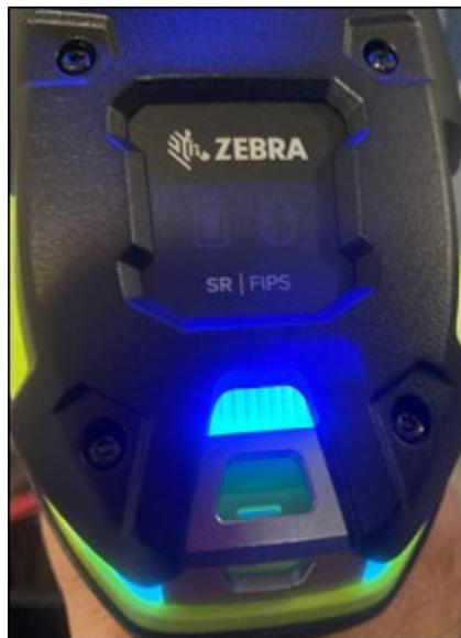
*Figure 3-23 – Paged scanner will glow Blue, Beep and vibrate 3 times.*
