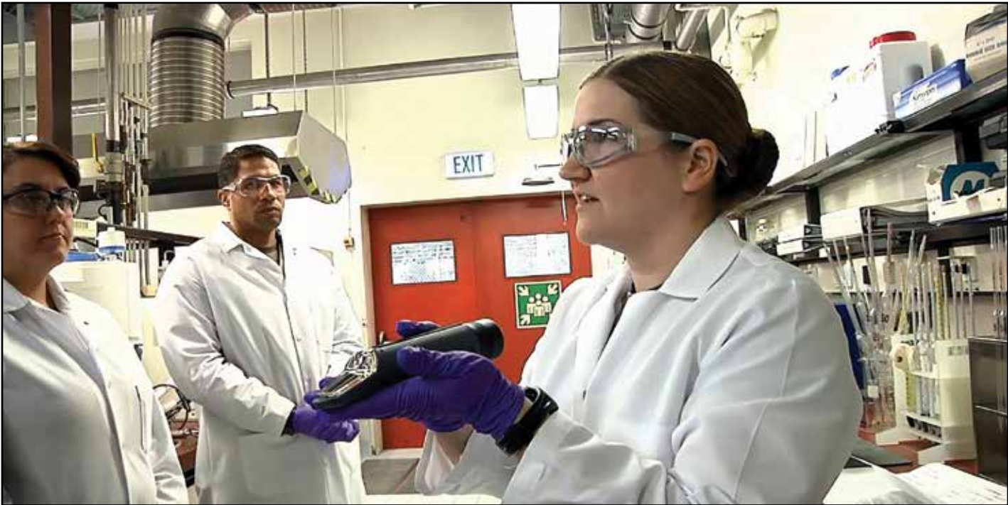
DLA Energy Europe & Africa Petroleum Laboratory noncommissioned officer in charge, Army Sgt. First Class Mandy Allen instructs 21st Theater Sustainment Command Soldiers on how to determine the fuel system icing inhibitor content of JP-8 jet fuel during the quarterly Fuel Handler's course. 21st Theater Sustainment Command Public Affairs photo
