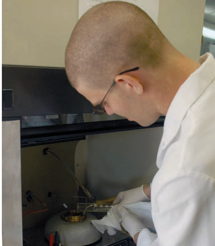
A soldier pours a fuel sample into a machine in his lab in Kosovo, that tests the flash point of the fuel. DLA Energy provides 50 percent of the fuel in Afghanistan, and 100 percent of the requirements in Europe and South America. Photo by Army Sgt. Jerry Boffen
