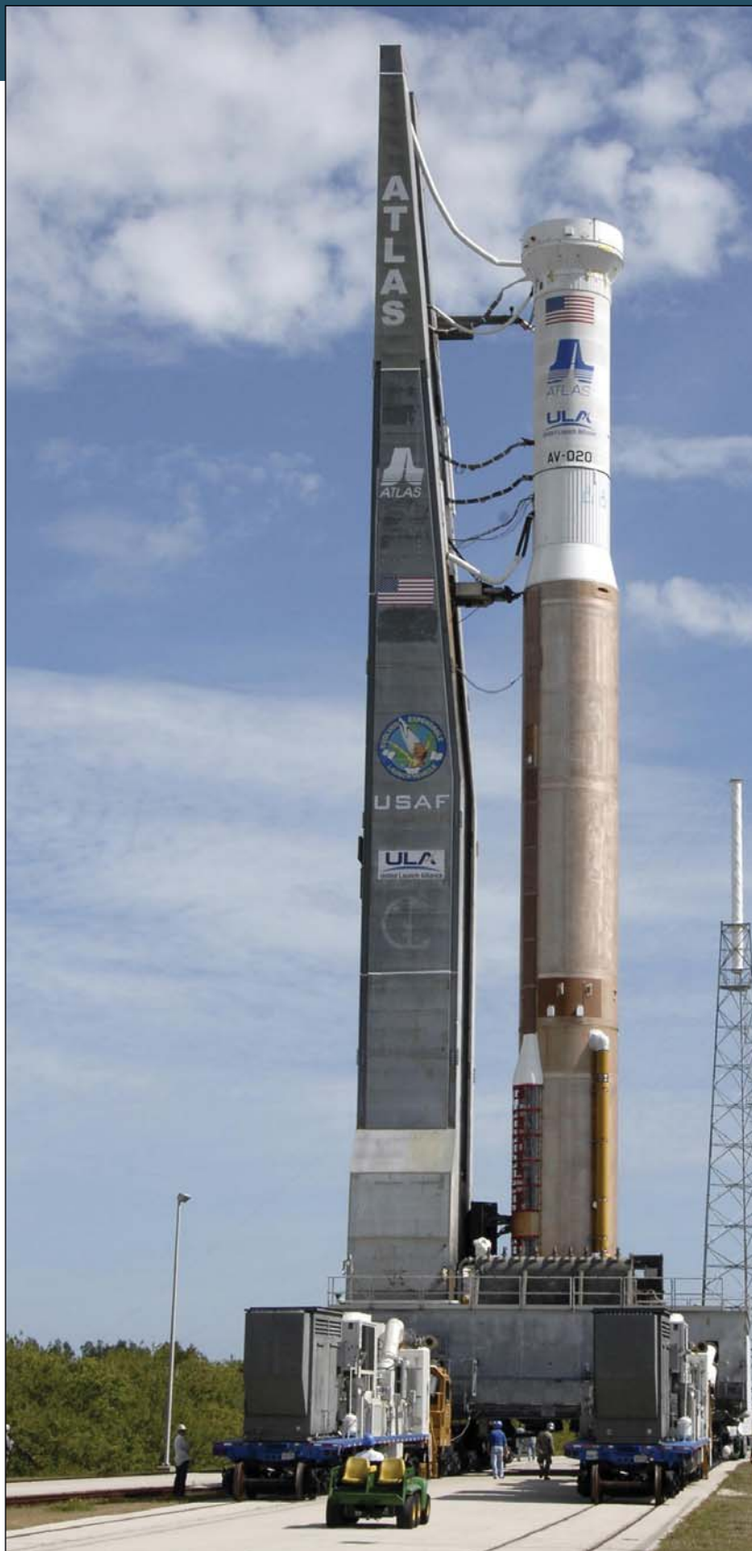
United Launch Alliance's Atlas V rocket is moved to the launch pad in preparation for a wet dress rehearsal at Cape Canaveral Air Force Station, Florida. During the rehearsal, the rocket was fully loaded with propellants, including liquid hydrogen, liquid oxygen and RP-1 fuel procured from the DLA Energy Aerospace Energy office. Photo by Kim Shiflett
