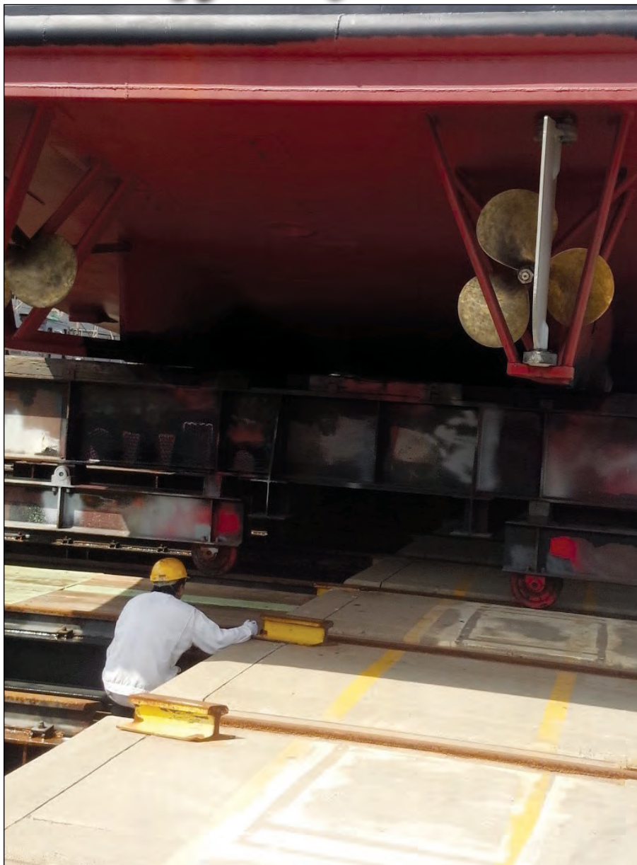
A Landing Craft Mechanized vessel undergoes repair work, including propeller restoration, installation of fuel gauges and parts, sandblasting and new primer (anti-rust) paint at the Shin-Itoman Ship yard in Okinawa. As the only DLA Energy-operated defense fuel support point in the Pacific, DLA Energy Pacific at Okinawa's mission is to support all Defense Department activities on Okinawa and to manage U.S. Pacific Command war's reserve fuel objective on Okinawa.
