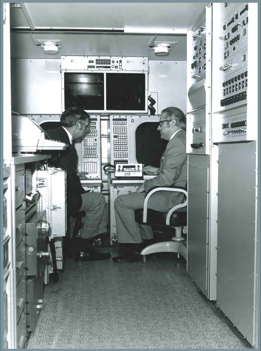
Specialists from Defense Contract Administration Region Los Angeles inspect the Army's Missile Minder, a transportable air defense fire control system, December 14, 1976. DCAR Los Angeles was one of the nine contract management regions DSA oversaw at the time. (DLA Photo)
