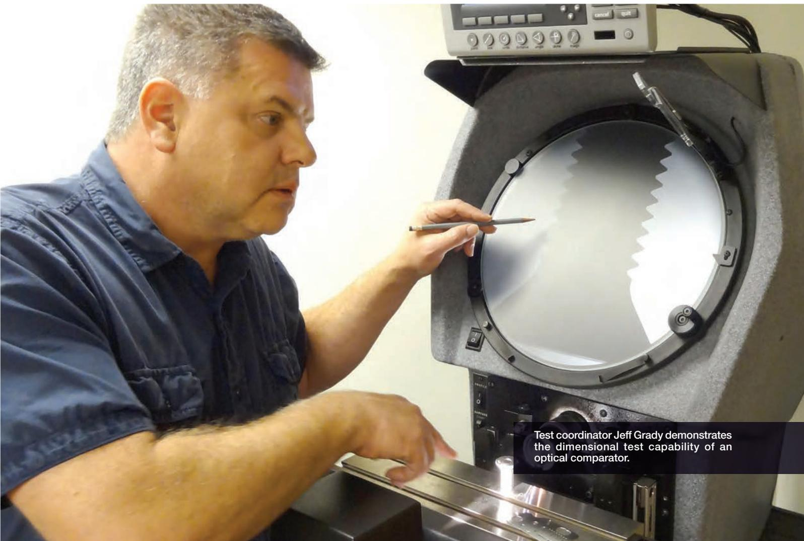
Test coordinator Jeff Grady demonstrates the dimensional test capability of an optical comparator.
