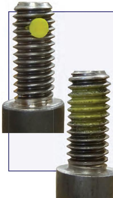
**Conforming bolt and nonconforming bolt; the conforming one contains the yellow self-locking pellet. The nonconforming one has a yellow spray mark.**
