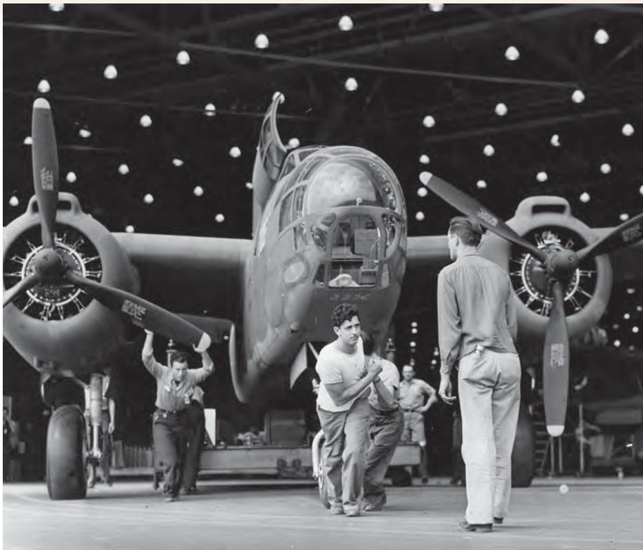
A Douglas A-20 attack bomber leaves the assembly line at the Long Beach, Calif., plant for transfer to the flight line and a test flight before delivery to the Army.
