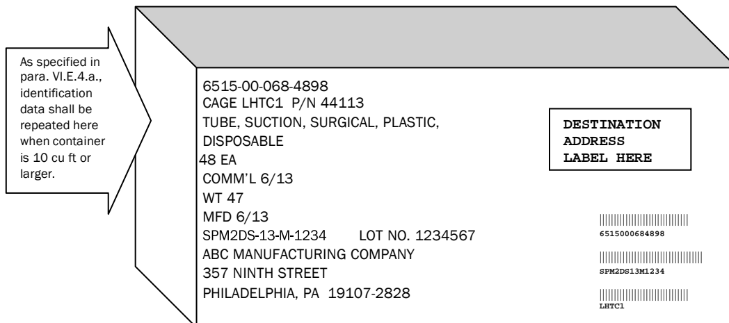
Figure 6. Exterior (Shipping) Container Optional Bar Code Placement All FSCs
