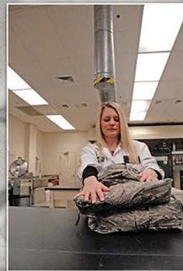
In this test, a lab specialist gauges the integrity of taped seams of the Air Force Environmental Parka for water permeability and appearance, before and after laundering.
