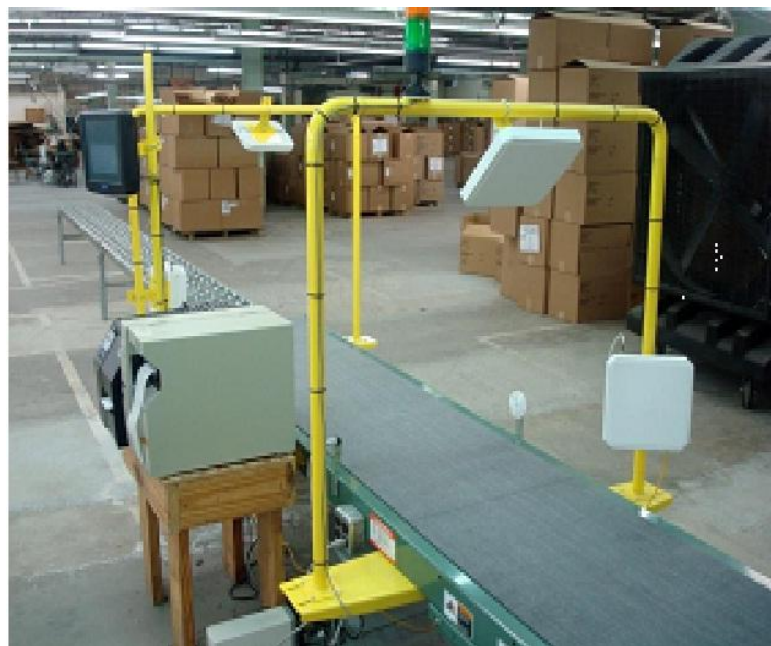
Figure 15. Conveyor with Fixed pRFID Readers
