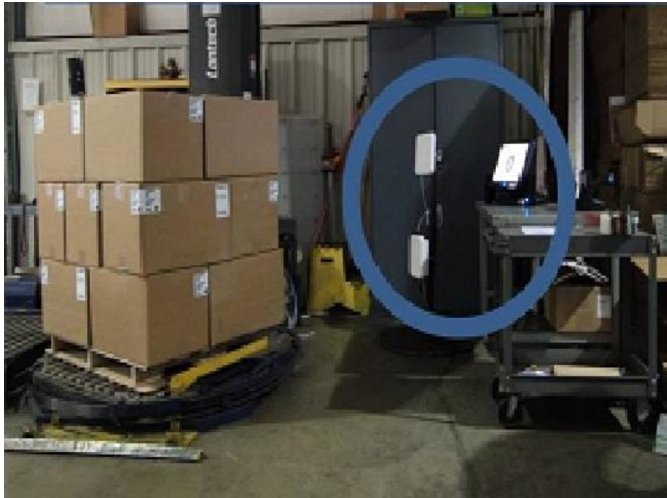
Figure 22. Linking Cases to Pallet—RFID-Enabled Palletizer
