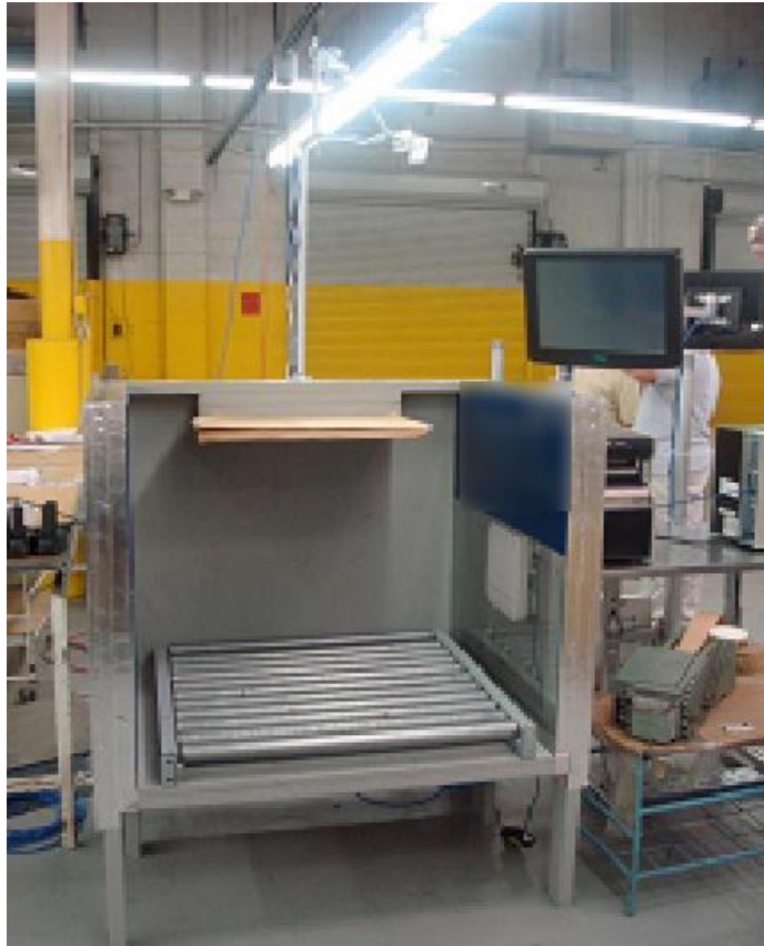
Figure 15. Conveyor with Fixed pRFID Readers
