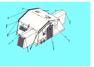
either a window or door on each sidewall. The roof panels feature either a stovepipe shield for a standard 4" stovepipe (temperate sections) or two large screened panels for extra ventilation (desert/tropical). Both have weather seal flaps. The liners have a bright white interior and a extra blackout lamination for a tactical environment. The roof fly helps shield the tent from the elements.
