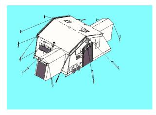
a window or door on each sidewall. The roof panels feature either a stovepipe shield for a standard 4" stovepipe (temperate sections) or two large screened panels for extra ventilation (desert/tropical). Both have weather seal flaps. The liners have a bright white interior and a extra blackout lamination for a tactical environment. The roof fly helps shield the tent from the elements.
