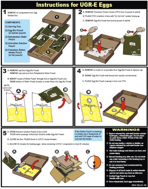
FIGURE 1. <u>BIB Module Operating Instructions, for Heater with Hydrogen Generating</u> <u>Warning</u>
