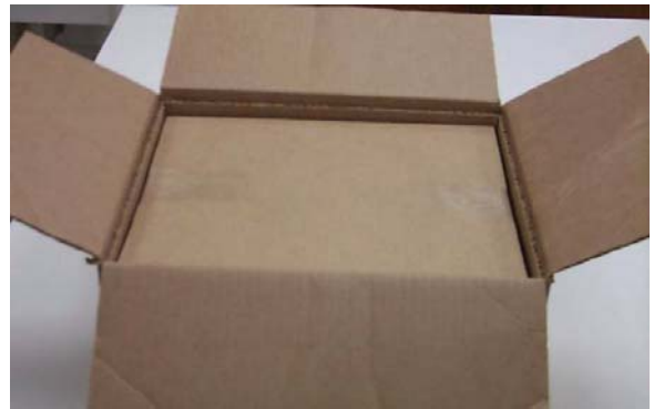
Improper Box & Liner Height Scored as Inadequate Workmanship
