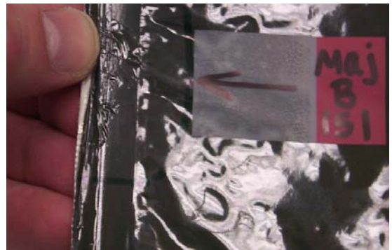
Outer- Ply Delamination - Propagated
