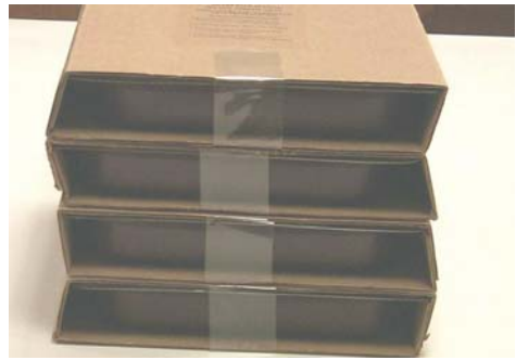
Improper Stack & Restraint Combo
