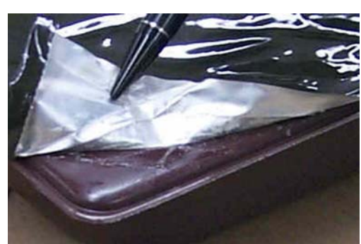
Leakage Under a Non-Cont. Seal
