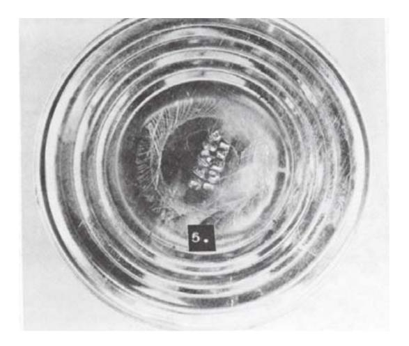
Table IV, Defect No. 204, Minor defect-scoring. (Disregard number on lid).
