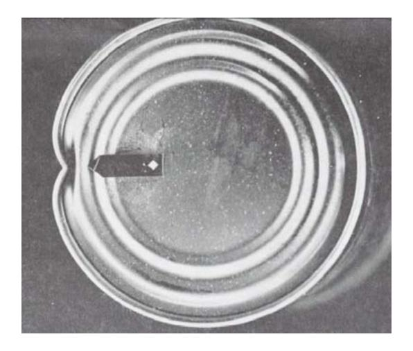
Table IV, Defect No. 110. Major defect. Severe end seam dent likely to affect the usability of the container.
