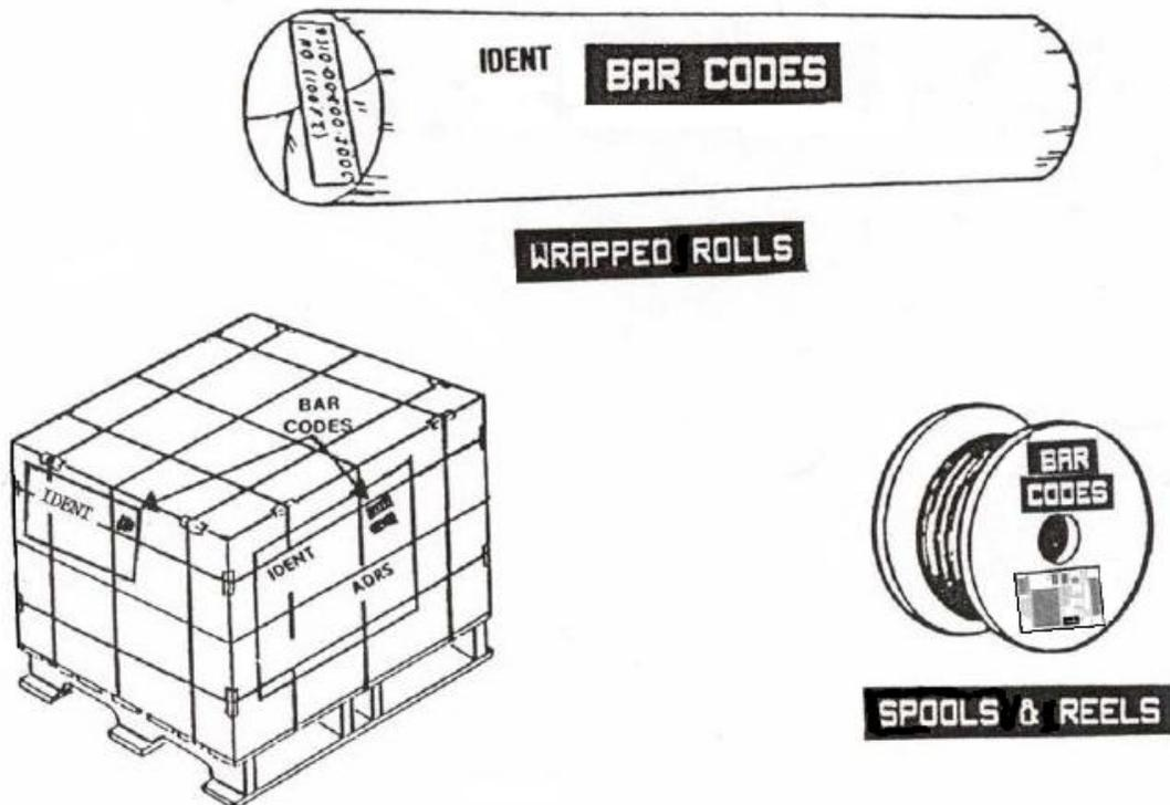
FIGURE 25. Bar code marking on miscellaneous materiel.
